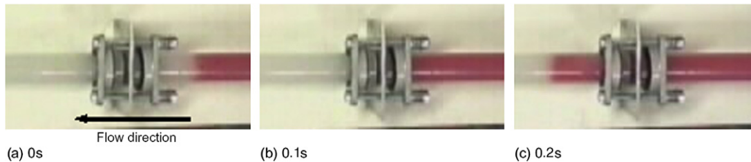
Fig. 5. Passage of 60% ice slurry through an orifice at a flow velocity of 0.4 m/s.
